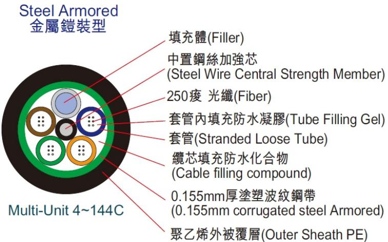
2~12 fibre per tube(Multi tube)
